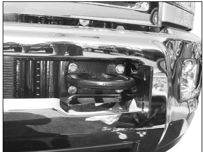
(Fig 4) Grille Guard Bracket mounted with factory tow hook. Use the supplied longer (8) 10mm x 45 Hex Bolts and hardware for installation
