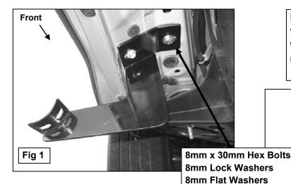
Remove the (2) plastic plugs or factory hex bolts to uncover the threaded holes in each mounting location.
