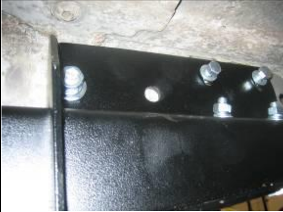
Driver Side Rear Mounting Bracket
