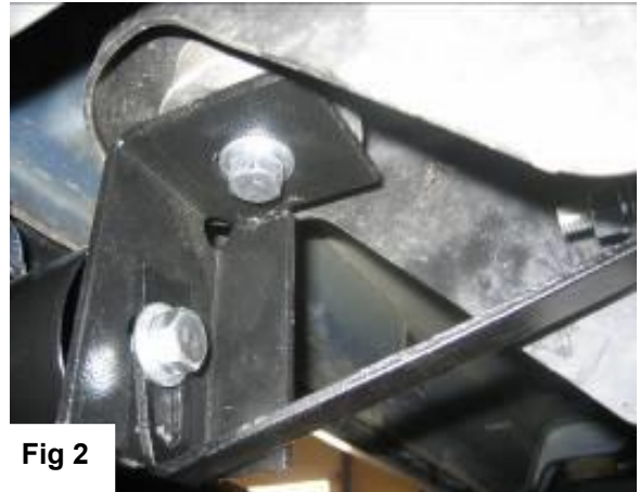
Passenger Side Front Bracket Installation
