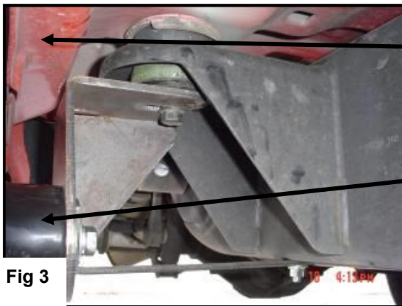
Passenger's Rear Bracket installation shown.
