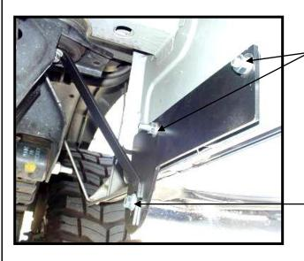
Attach rear bracket to inside of rocker panel using (2) 3/8" bolt plates, (2) 3/8" flat washers, (2) 3/8"lock washers, and (2) 3/8" hex nuts.
