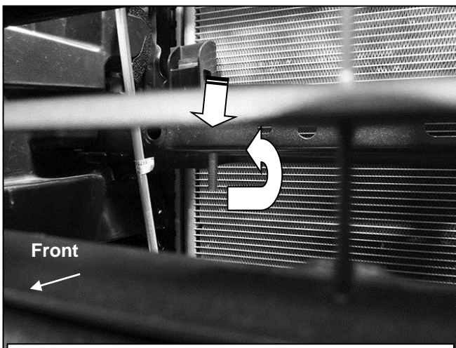
(Fig 9) Insert Bolt plate (arrow) into back of radiator cross support and down through hole in bottom (passenger side pictured through bumper)
