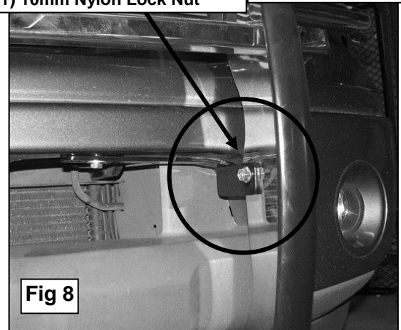
05-08 driver side Top Bracket installation pictured
