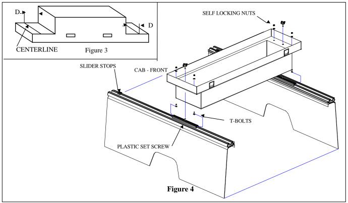
12) Slide the Toolbox Mounts onto the inner Top T-Track of each Base Rail, approximately 24"from tailgate. Starting with the driver's side, insert the Square Nut into the Slider's Top Slot, and position it over the selected hole for the Knob. (see step 8) Thread the 1" Plastic Set Screw through the Nut into the Slider. (**Do not bottom out screw into Base Rail.**) Repeat on passenger side. (Figure 4)
