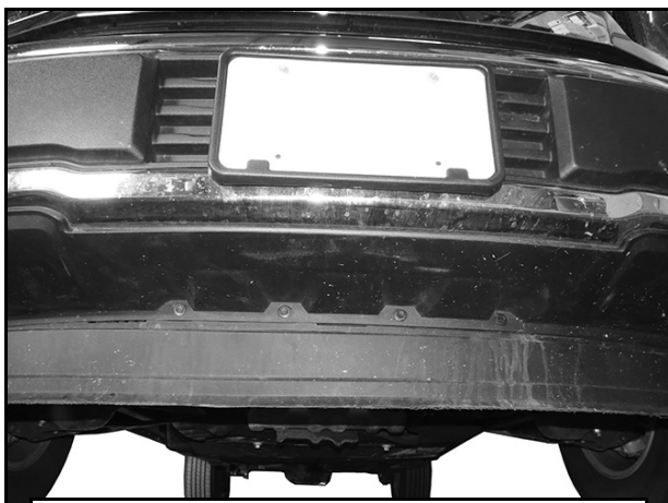
(Fig 1) Remove license plate from Bumper
