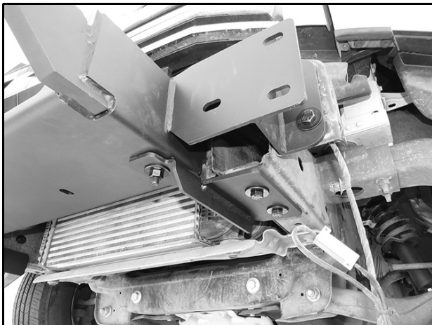
(Fig 13) Driver/left Support Bracket installed
