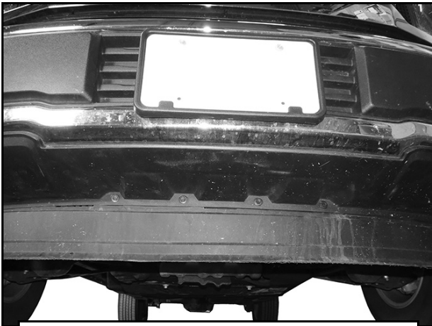
(Fig 1) Remove license plate from Bumper
