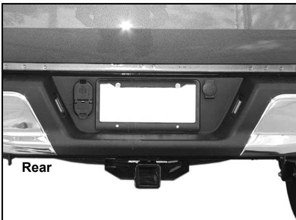
(Fig 1) Unplug and remove 7-wire trailer plug
