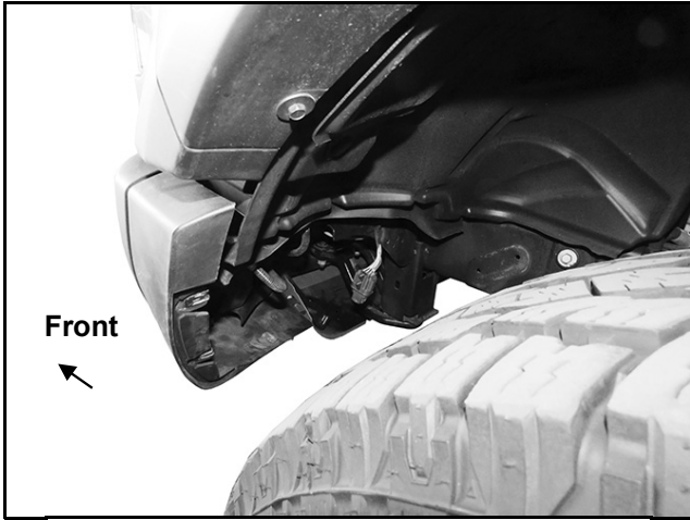
(Fig 1) Remove lower fender liner. Unplug wiring harness leading to front bumper
