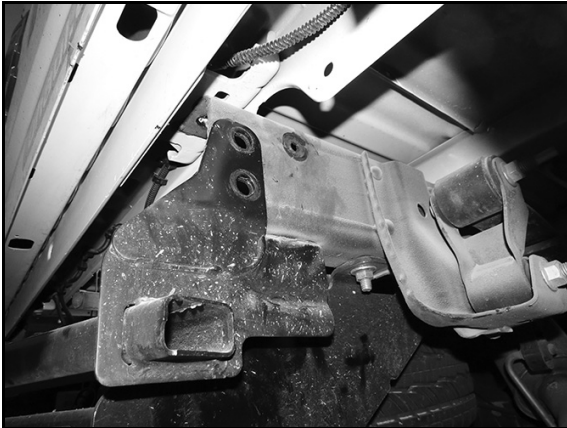
(Fig 5) End of frame once bumper is removed. Passenger/right side with receiver hitch
