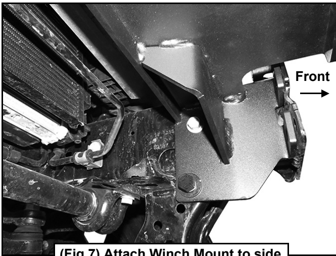
(Fig 7) Attach Winch Mount to side of frame (driver/left side pictured)
