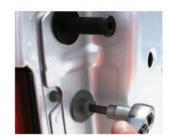
Step 7: Install the bolt removed from the previous step through the hole in the ball mount plate back into the hole.
