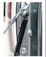
Install the narrow end of the shock on the ball mount
