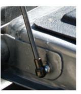
Periodically check the upper and lower mounting locations to ensure that parts have no loosened from repeated use. If either mounting location is found to be loose, re-tighten the hardware as needed.
