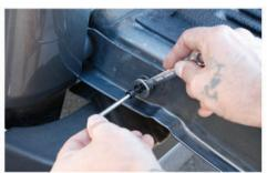
Warning: Overtightening the nutsert can strip the threads and cause the nutsert to be nonfunctional.
