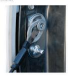
Tighten the bolt with the T-50 Torx socket.
