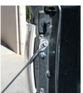
Step 6: Install the cable back on the cable bolt and the larger part of the shock on the ball mount.
