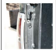
Step 5: Install the bolt removed in the previous step through the hole in the ball mount plate back into the hole. Tighten the bolt with the T50 torx socket.
