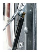
Step 7: Install the narrow end of the shock on the ball mount that was just previously installed.
