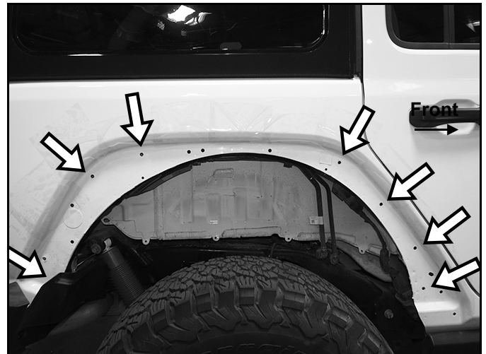
(Fig 4) Drill 25/64 hole in body panel at (7) locations (arrows). NOTE: These locations are not accessible from back of body panel
