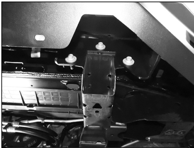
(Fig 12) Attach the Bumper to Frame Bracket
