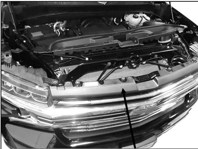
(Fig 1) Remove cover and screws attaching grille
