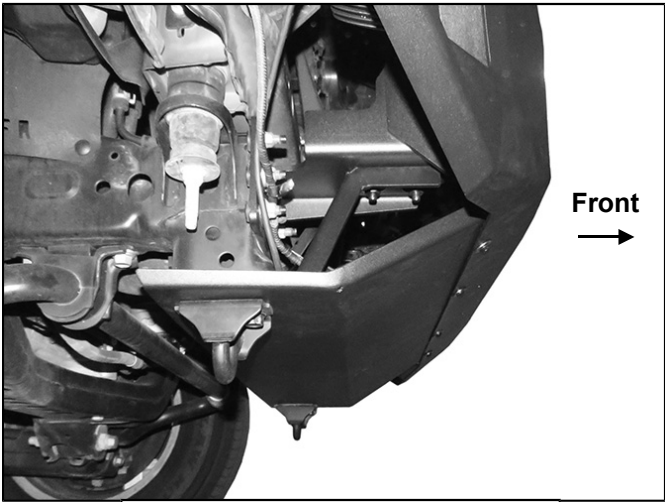
(Fig 4) Skid Plate fully installed
