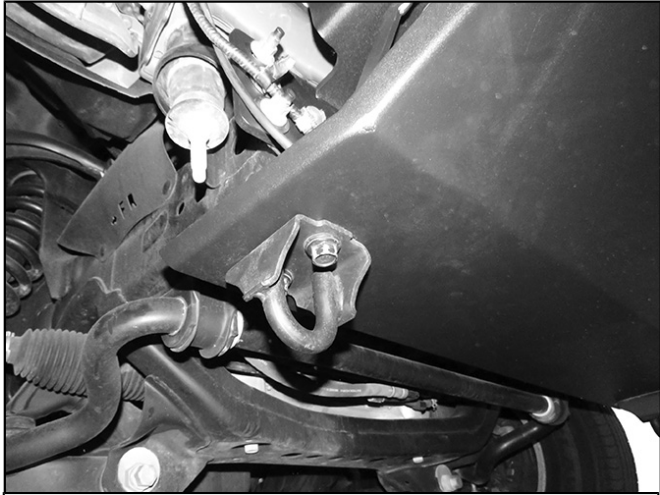
(Fig 3) Reuse tow hook and hardware to attach back of Skid Plate to Support Bracket and frame
