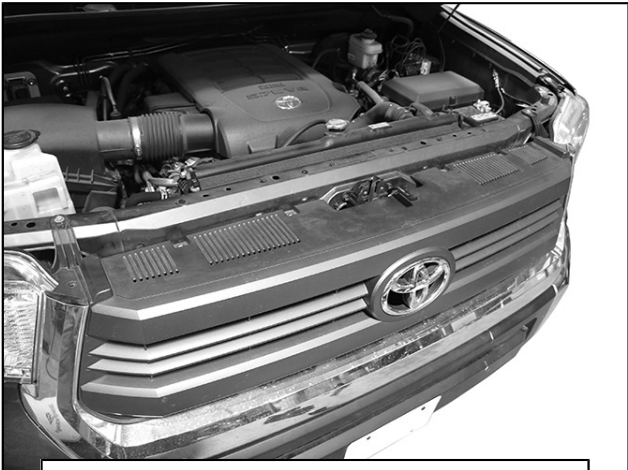
(Fig 7) Remove plastic cover and grille for access to bumper bracket hardware
