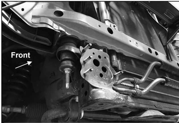
(Fig 8) Passenger/right side frame mounting location (bumper & grille removed)
