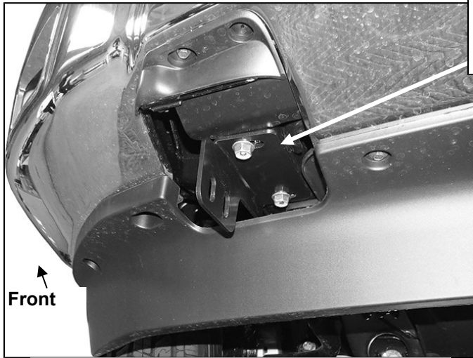
(Fig 5) Non-tow hook models, attach Frame Mounting Bracket directly to bottom of frame
