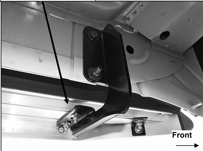
(Fig 8) Driver/left front Bracket installed
