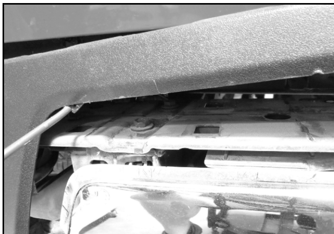
(Fig 6) Remove factory hardware under the plastic cover attaching bumper to top and bottom of hitch
