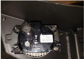
Install the factory foglight to the foglight mount using the (4) M4 allen bolts, washers and nuts. (For JK, JL Sahara and JL Rubicon Versions)
