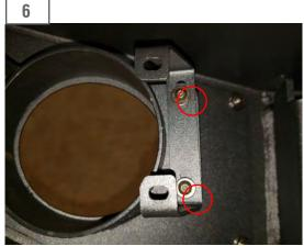
Install the (2) LED fog light brackets to the fog light mounts of the bumper using the (4) M4 allen bolts, washers and nuts.
