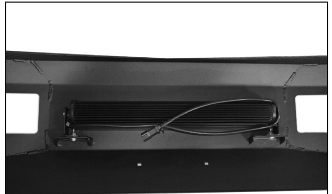
(Fig 7) Center LED light bar installed (pictured from behind the Bumper)
