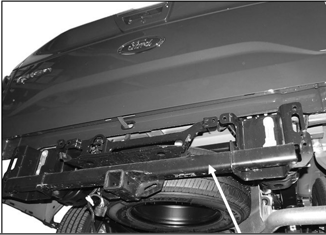
(Fig 15) Reinstall integrated receiver hitch/bracket assembly on models with "HD Towing" package
