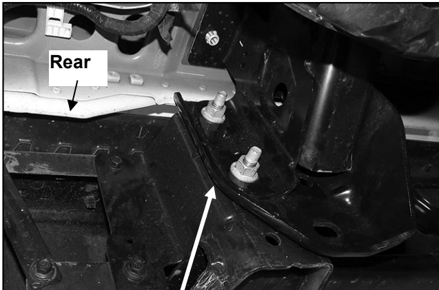
(Fig 3B) Remove the factory hex nuts attaching bumper assembly to frame. STD tow package model pictured (no receiver hitch)
