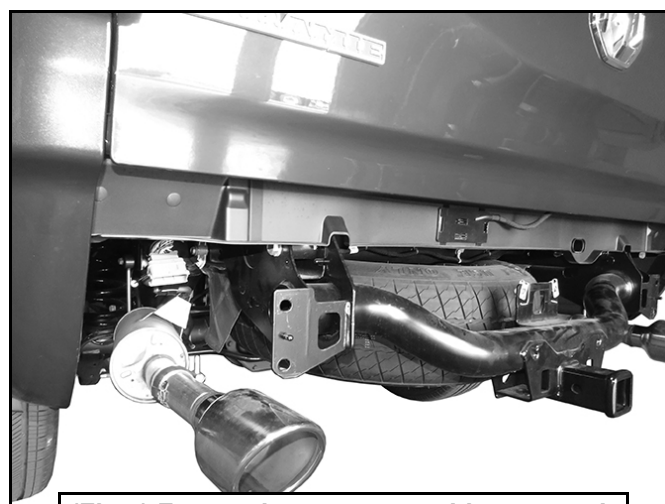
(Fig 4) Factory bumper assembly removed
