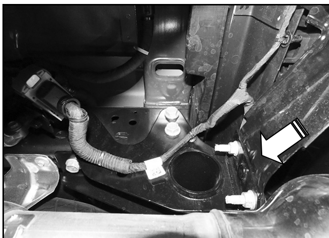
(Fig 3) Remove hex nuts to remove bumper (arrow)
