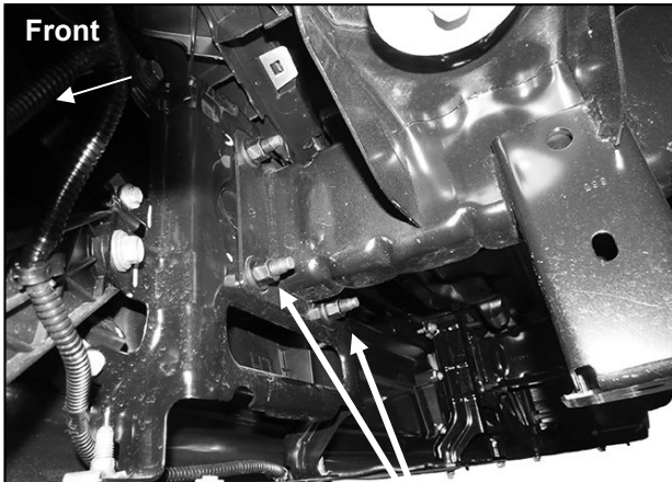
(Fig 5) Remove (3) factory hex nuts from each side
