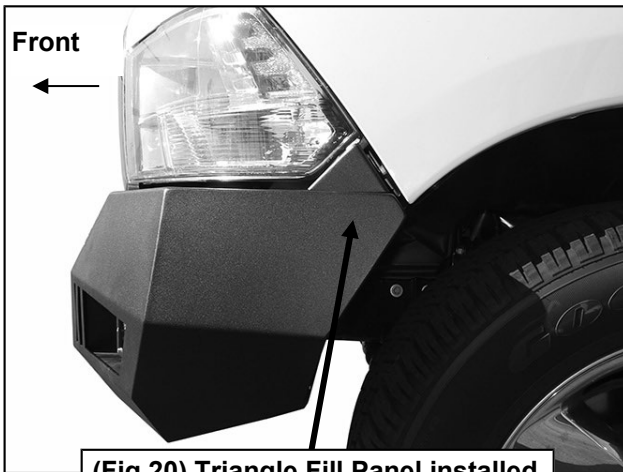
(Fig 20) Triangle Fill Panel installed
