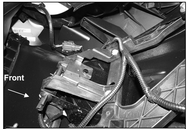
(Fig 2) Unplug fog lights if equipped. Unplug harness to bumper and move harness
