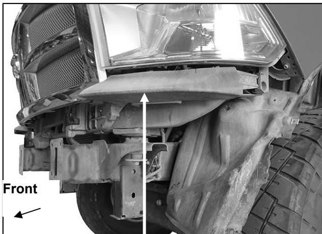
(Fig 7) Remove plastic block from below headlights
