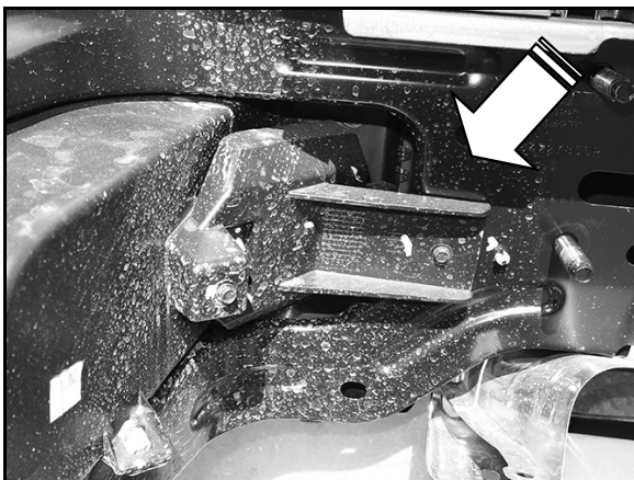
(Fig 9) Remove the cross traffic sensors if equipped (arrow)
