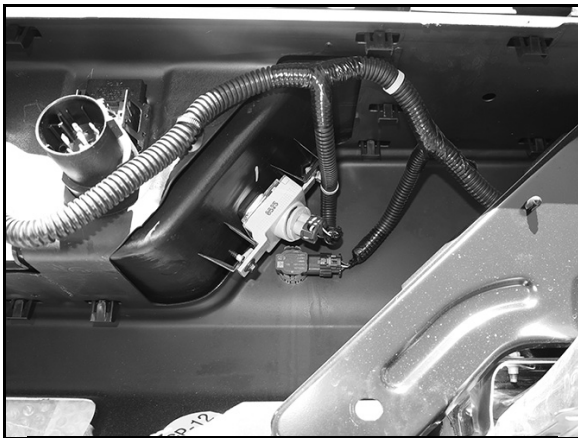
(Fig 7) Remove the license plate lights, the trailer plug and wiring harness
