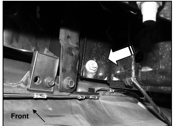
(Fig 10) Models without tow hooks, loosen the front hex nuts to tilt the bumper enough to insert the Double Nut Plates into the end of the frame. Remove factory hex nut (arrow) from back of bumper bracket and tilt bumper forward
