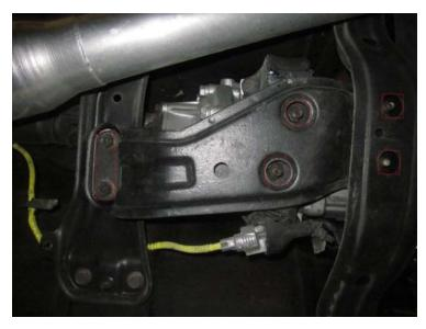
3. Remove the Transmission crossmember by dropping the back down and
