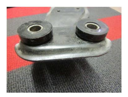
8. Reinstall crossmember and torque all bolts to 27ftlbs
