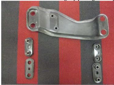
6. Remove the dowel pins from the old bushings and install them into the new bushings. Take note that 4 of the bushing have a lip to them and the other 4 do not.
