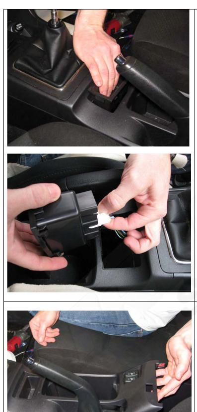
**3.** Remove the small storage compartment in front of the handbrake by pulling up on it as pictured to the left.
