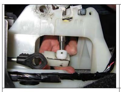
**26.** Re-connect the lower shifter cable to the shifter. If you left the steel clip in place on the shift cable, the cable can simply be pressed on to the plastic pivot cup until the steel clip snaps in to place. Lower the short shifter in to place making sure the bottom rectangular pivot cup with the o-ring is seated properly in the shift assembly.
