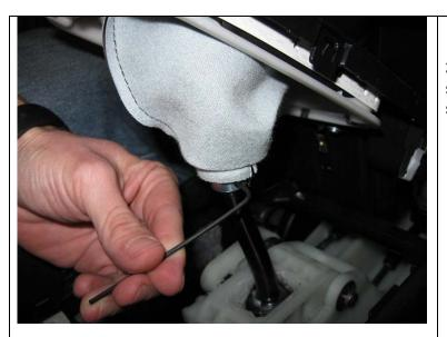
**38.** ...continued. Pictured to the left is the special shift boot retainer secured to the shifter.
