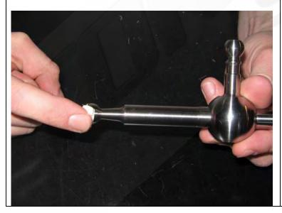
**22.** Grease the small ball on the bottom of the short shifter as shown at left.Torque Solution recommends using white lithium based grease, however any automotive grade grease will suffice.
