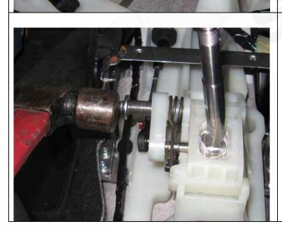
**28.** Re-install the top white plastic cap and the triangular shaped side arm. Be sure the shifter is properly seated in the bottom pivot cup, and that the side arm spring pivot is inserted in to the spring. Now re-insert both of the pins which secure the top white plastic cap. It may be necessary to lightly tap them through the assembly with a hammer to be sure they are fully inserted through the assembly.
