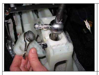
**20.** The plastic triangular side arm and spring can now be removed from the shift assembly. The shifter can now be pulled up and out of the shift assembly. Pay close attention to how the spring is installed on the side arm as you will have to re-install it later.
