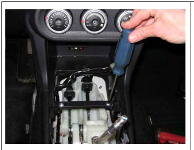
**10.** Use a Phillips head screwdriver to remove the 2 screws in front of the shifter that have been exposed by removing the front portion of the console in the previous step.
