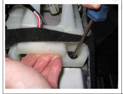
**32.** Lift the shift assembly slightly and use a flat head screwdriver to push the steel sleeves in the rubber bushings out through the bottom of the bushing. Repeat for all four corners.
