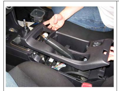
**5.** The front portion of the rear half of the console can now be lifted and separated from the rest of the console. It is held in place by clips from underneath so it will pop free by lifting upward.
