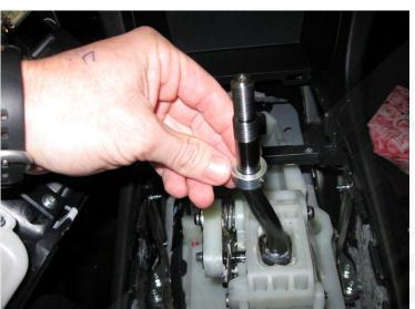
**36.** Re-install the center console and reconnect all wires and connectors by reversing steps 10 to 13. Install the special shift boot retainer on the shifter as pictured to the left. Do not tighten the set screw yet.
