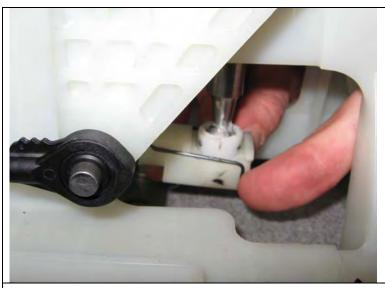
**14.** Working at the bottom of the shifter itself, spread the steel wire clip apart with your fingers or needle nose pliers and push the cable down. This will separate the shifter from the shifter cable. Be sure not to lose the steel wire clip as it needs to be used for reinstallation.
