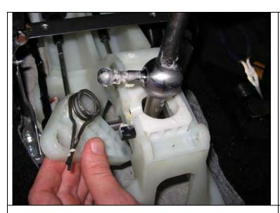
**20.** The plastic triangular side arm and spring can now be removed from the shift assembly. The shifter can now be pulled up and out of the shift assembly. Pay close attention to how the spring is installed on the side arm as you will have to re-install it later.
