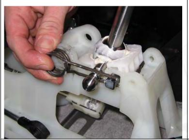
**27.** Re-install the spring for the triangular shaped side arm ensuring it's orientation is correct as pictured to the left.
