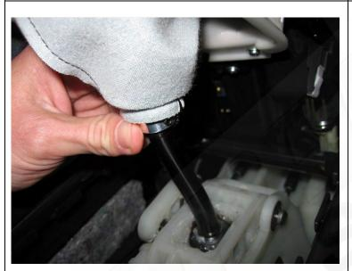
**38.** Lift the shift boot and front part of the console as pictured to the left. Move the shift boot retainer up the shifter shaft so it holds the top of the shift boot pressed up against the bottom of the shift knob. You can now tighten the set screw to secure the shift boot retainer on the shifter with the supplied allen key.
