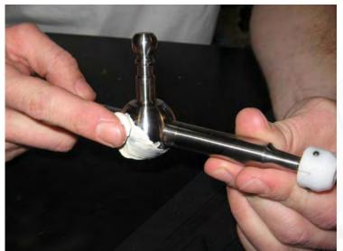
**24.** Grease the main pivot ball on the short shifter, as well as the small pivot ball on the side arm.
