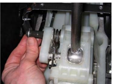
**18.** Take note of the orientation of the spring on the side of the shifter for re-installation later. Both pins that go through the shifter can now be completely removed from the assembly.
