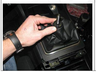
**37.** Install the front part of the console with the shift boot over the short shifter. Do not clip the console in place or re-connect the wire beneath it yet just slide the shift boot on to the shifter at this time.
