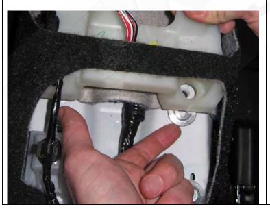
**34.** Install the base bushings beneath the shift assembly with the smaller diameter step facing up. This step fits in to the holes in the plastic assembly to replace the rubber bushings you removed in the previous step. Install a bushing at each corner of the shift assembly and ensure that the assembly is seated properly with each smaller diameter step on each bushing fully inserted in the holes at each corner of the assembly.
