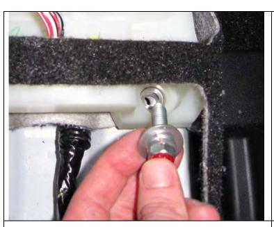
**35.** Secure the shift assembly back in place with the stock bolts and a 12mm socket and ratchet. Be sure the step on the bushings at each corner of the assembly are in the holes in the assembly properly before tightening it down.
