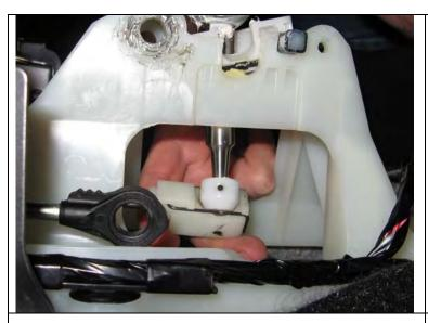
**26.** Re-connect the lower shifter cable to the shifter. If you left the steel clip in place on the shift cable, the cable can simply be pressed on to the plastic pivot cup until the steel clip snaps in to place. Lower the short shifter in to place making sure the bottom rectangular pivot cup with the o-ring is seated properly in the shift assembly.
