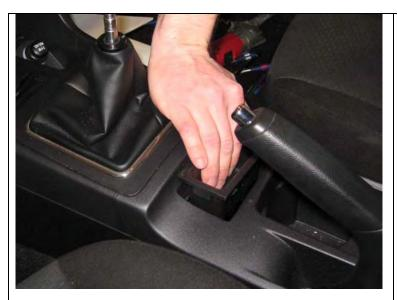
**3.** Remove the small storage compartment in front of the handbrake by pulling up on it as pictured to the left.
