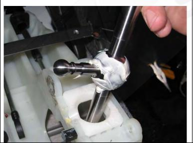
**25.** <u>Install the greased short shifter</u> in to the shift assembly.
