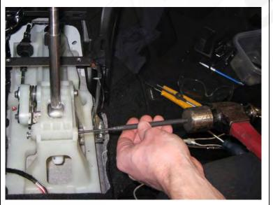
**17.** With the 2 clips removed and side shifter cable disconnected, push the two pins out of the assembly using a hammer and a small punch. Use a screwdriver if a punch is not available.
