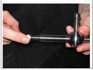
22. Grease the small ball on the bottom of the short shifter as shown at left. Torque Solution recommends using white lithium based grease, however any automotive grade grease will suffice.
