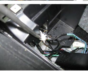
Begin by prying off the accessible part of the white tab as shown to the left. You can then access the opposite side of the tab hidden underneath the console. Use you finger tips to remove the other side of the tab from under the center console.
