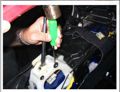
16. In order to remove the shifter, the 2 push clips on the passenger side of the shifter assembly holding the two pins must be removed or cut with a rotary tool or Dremel. If you do not have access to rotary tool, use a sharp flat head screwdriver and a hammer and work your way around the push nut to remove it. New push nuts are provided in the kit if they are broken or cut during removal.
