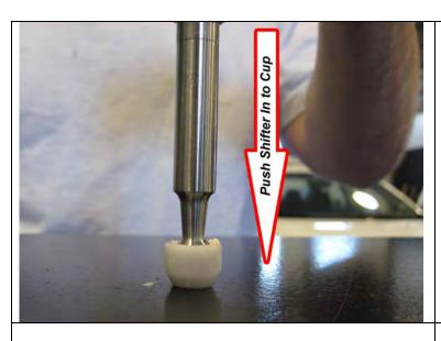
**23.** Press the small white cup you removed in the previous step on to the short shifter. Place the cup on a flat surface and push the shifter down in to it.
