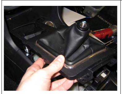
**7.** The front portion of the console with the shift boot attached can now be lifted, however it cannot be removed from the car yet as there is a clip holding a wire at the front which must be removed as shown in the next step.
