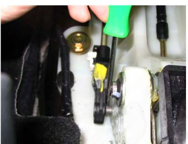
**15.** Disconnect the shifter cable that controls side to side motion from the triangular plastic side arm. This can be achieved simply by prying with a flat head screwdriver to slide it off the pin on the triangular plastic side arm.
