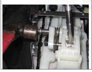
28. Re-install the top white plastic cap and the triangular shaped side arm. Be sure the shifter is properly seated in the bottom pivot cup, and that the side arm spring pivot is inserted in to the spring. Now re-insert both of the pins which secure the top white plastic cap. It may be necessary to lightly tap them through the assembly with a hammer to be sure they are fully inserted through the assembly.
