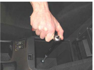
**12.** Open the storage compartment on the rear center console. Use a 10mm socket and a ratchet with a long extension to remove the 2 bolts in the bottom of the storage compartment.
