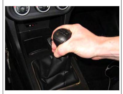
**1.** Unscrew the shift knob by rotating it counter-clockwise and put it in a safe place.
