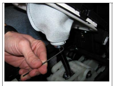
**38.** ...continued. Pictured to the left is the special shift boot retainer secured to the shifter.
