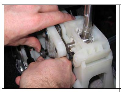
**29.** Re-connect the shifter cable that controls side to side movement to the pin on the triangular shaped side arm. It can be pressed on by hand.
