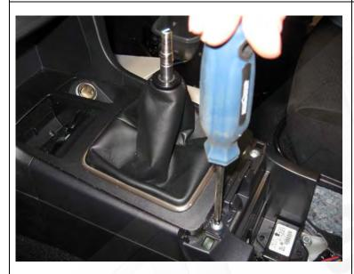
**6.** Use a Philips head screwdriver to remove the 2 screws directly behind the shifter.
