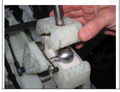
**19.** The white plastic cap can now be removed from the shift assembly. Put it in a safe place for re-installation later.
