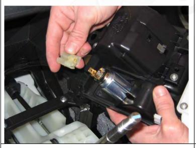
**9.** Turn this portion of the console over and disconnect the plastic plug for the lighter by pulling on the plastic portion. Do not pull on the wires. There are no tabs to depress on this clip, the connector simply slides off. The front portion of the console can now be removed from the car and put in a safe place.
