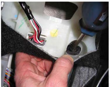
**33.** Remove the rubber bushings from the base of the assembly by pushing them down through the assembly with a flat head screwdriver or with your fingers. It is helpful to pull on the bushings from beneath the assembly with your fingers while pushing them down through the top with your other hand. Repeat for all four corners of the shift assembly.
