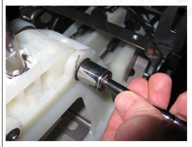
**30.** Secure the pins in the assembly with the supplied push clips. Use a 14mm socket to install the 10mm push clip on the larger pin at the front of the assembly by driving it on with a ratchet extension.
