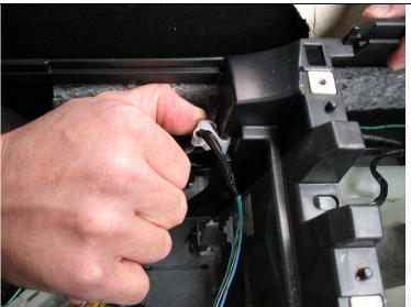
11. In order to remove the center console, you need to disconnect the white tab holding wires to the console as shown to the left. You can pry off the white tab from the black tab by using a flat head screwdriver.
