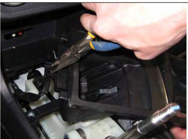
**8.** Use needle nose pliers to compress the tabs on the clip at the front part of this section. With the tabs depressed, the clip can be pushed through and out from the under side.
