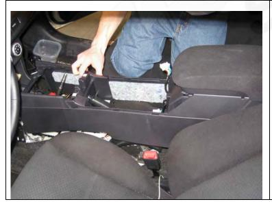
**13.** The center console is now free and can be removed from the car. Put the console in a safe place for re-installation later.
