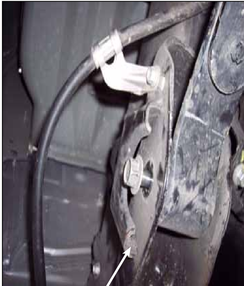
Factory bolt backed out 1/2"
