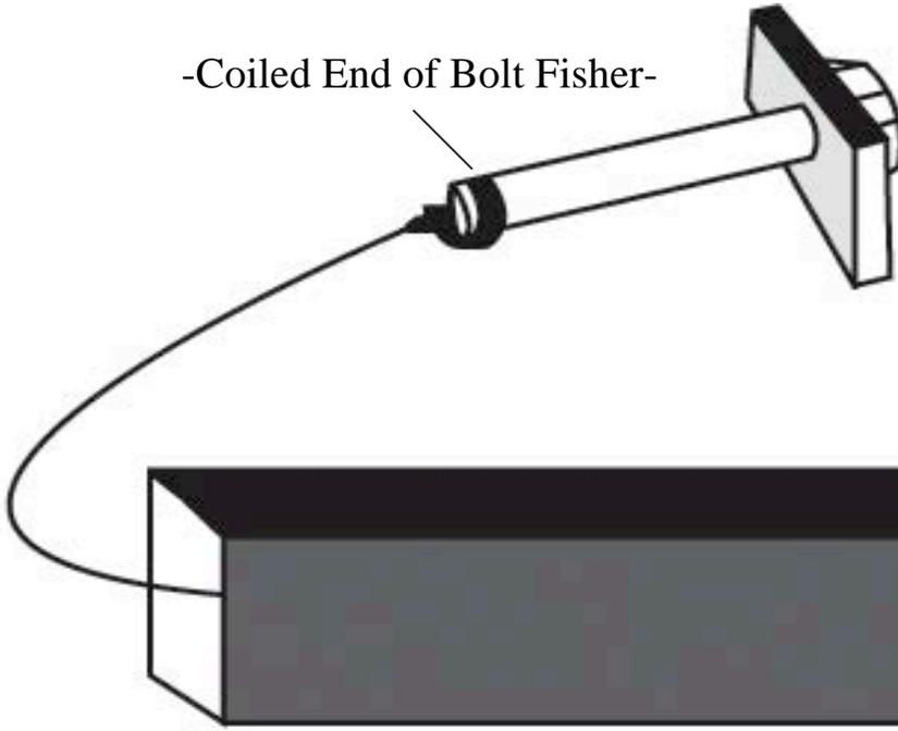
Note: The hardware may vary as to what is being fished along with the bolt. In this instance a 1”(2cm) X 2”(5cm) plate washer is being fished along with the hex bolt. Different applications may require fishing through various star washers and flat
