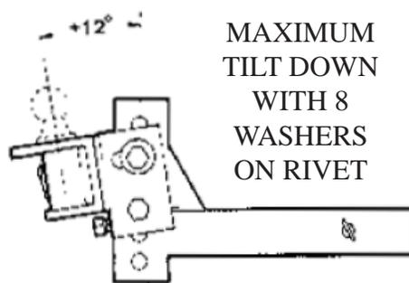
MAXIMUM TILT DOWN WITH 8 WASHERS ON RIVET
