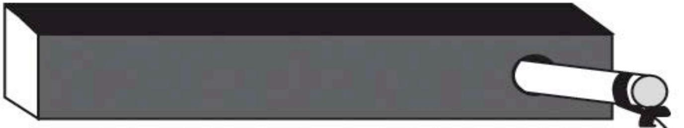
This bottom example shows the bolt when it's completely fished through the vehicle. You may find it easier to keep the bolt fisher attached until you get the tie down receiver in place so that the bolt doesn't fall into the vehicle frame.
