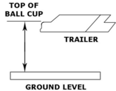
2. After ball height has been determined write down the ascertained height. EXAMPLE: Measured top of coupler height was 17" (43cm) from ground; ball height should be 18 1/2" (47cm).
