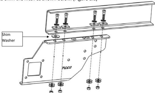
Now the eight frame bolts can be re-tightened. Starting from the rear of the
