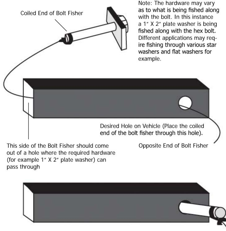
This bottom example shows the bolt when it's completely fished through the vehicle. You may find it easier to keep the bolt fisher attached until you get the tie down receiver in place so that the bolt doesn't fall into the vehicle frame.
