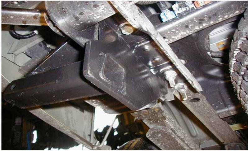
**NOTE:** Short bed trucks will use the two factory bolts that currently attach the corner bumper brackets to the frame (**SEE PHOTO BELOW**). Loosen the corner bumper support bracket at the bumper (both the upper and lower fastener) as this will allow the corner bracket to hinge out from the frame after removing the two nuts which attach the corner bracket to the frame.
