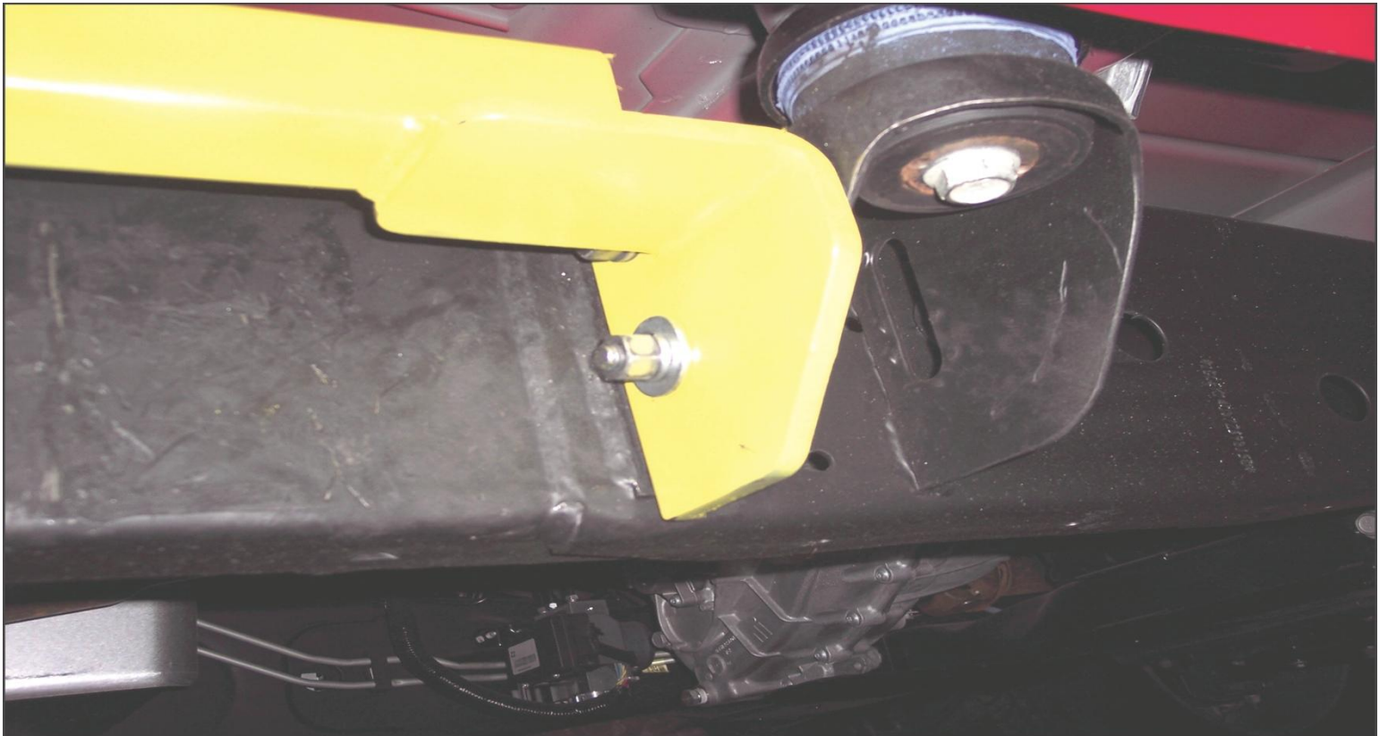
Completed Passenger Tie down
