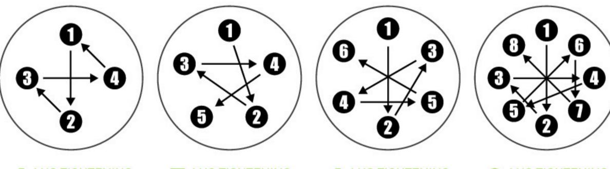
LUG TIGHTENING 5 LUG TIGHTENING PATTERN **4** PATTERN
