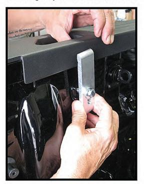
**STEP 2:** Insert 1/2 of the rear clamp into the stake pocket. (clamp w/ 2 flat grips)
