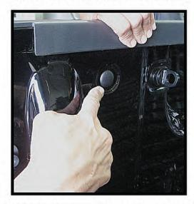
**STEP 3:** Position the longer clamp bracket w/ plastic insert and aling to inner bracket. conect both using the provided bolt and washers.
