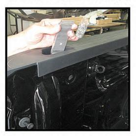
STEP 4: Install the Aluminum Side Rail starting at the front using the smaller clamps provided. Slide the Side Rail into the rear clamp system. Continue Following Standard Installation Instruction Manual.
