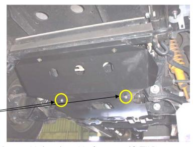
Remove original guards, retaining fasteners, and fit TJM Front Underbody Guard using original fasteners plus the fasteners supplied.
