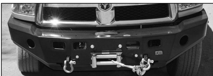
In this picture RHS of bumper wing tip is 1/8" below bottom of body – on level ground it is 7/8" below. This is due to body to chassis twisting in rubber body mounts.
