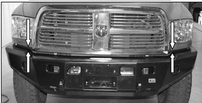
Maintain equal distance from these points around to tips of wings both sides.
