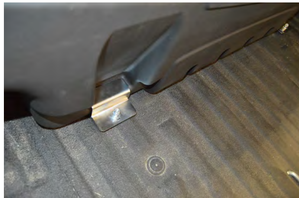
(Fig. 11) Toe clamps installed on Mounting Brackets
