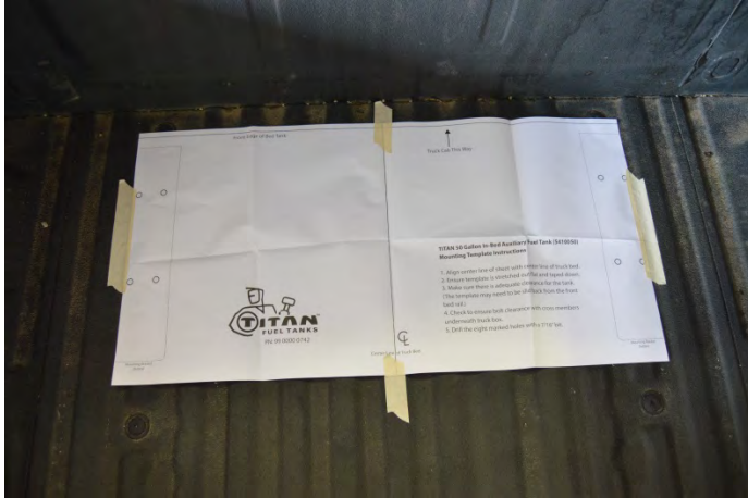
(Fig. 4) Template for drilling mounting holes taped down.
