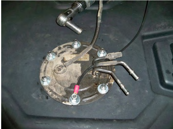
(Fig. 4) Be sure to attach Grounding Wire to one of the studs holding the sending unit.
