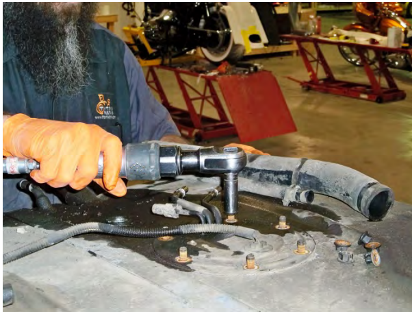
(Fig. 1) Loosen the bolts holding the sending unit into the OEM tank.
