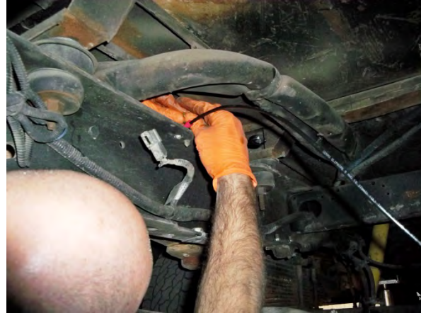
(Fig. 5) The other end of the Grounding Wire must be attached to a bolt on the vehicle frame.
