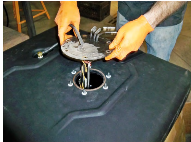
(Fig. 2) Carefully place the OEM sending unit into the new TITAN™ replacement tank.
