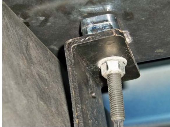
(Fig. 12) Tighten the bolt and bracket against the shims. If the strap does not hold the tank tightly enough, remove one shim at a time until it is tight.
