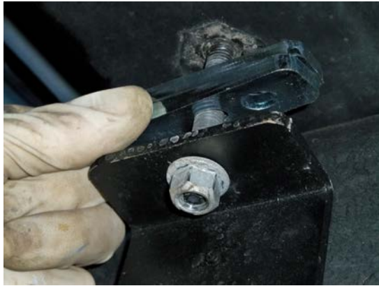
(Fig. 11) If included, thread two shims onto each strap bolt. In the case of GM, thread bolt up through strap and shims.
