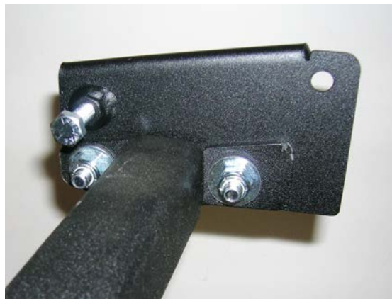
(Fig. 13) Shown: Right Hand Bracket for GM Cross Bar. The Cross Bar is held fast by tightening the 5/16" cap screw seen here at the upper left hand corner of the bracket. In severe applications it is recommended that the installer position the Cross Bar, mark the center of this cap screw hole, drill a hole in the front lip of the frame and then tighten the cap screw into the hole. It is advisable to apply Loctite Threadlocker or equivalent to the bolt. By early 2009, TITAN will be shipping a "Super Series" bracket with each tank as shown above. In a severe application, using this bracket, the installer may position the bracket, tighten down the cap screw as shown, and then drill a hole in the frame lip through the hole seen in the right hand corner of the bracket. An extra 5/16" cap screw and nylon locking nut are provided for fastening this extra hole.
