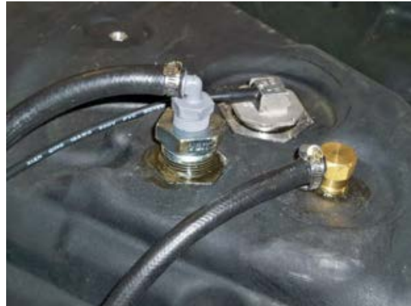
(Fig. 7) Install 5/16" hose onto the rollover valve
