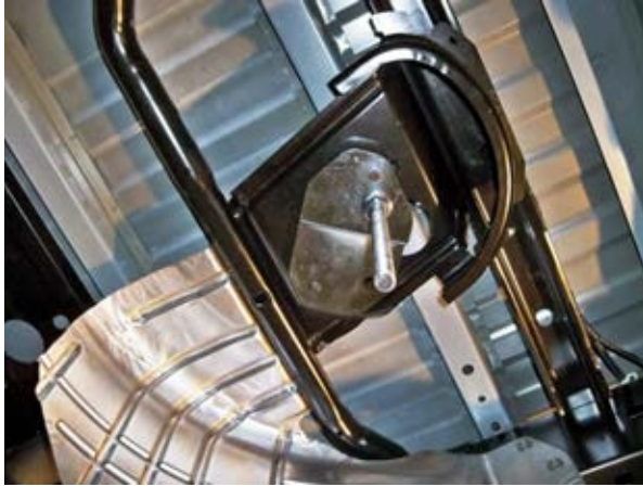
(Fig. 2) Cross member in 2013+ RAM vehicles showing STAFS top Truck Mounting Plate and Threaded Rod installed.
