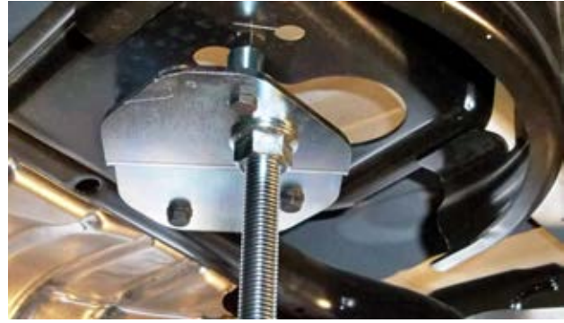
(Fig. 3) Cross member in 2013+ RAM vehicles showing STAFS Truck Mounting Plate close-up.
