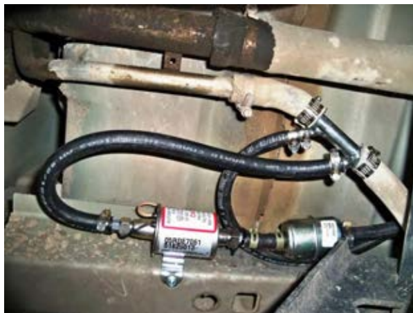
(Fig. 15) Vent Fill Neck Adapter installed.
