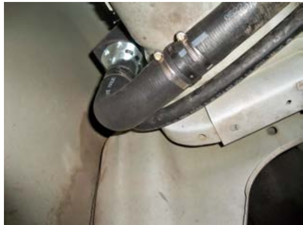
(Fig. 18) Check to be sure there is room in the fender space for the Poly Fuel Neck Flange Assembly BEFORE cutting any holes. Always test fit FIRST. Some fender spaces may require the trimming of sheet metal components to allow proper fit.
